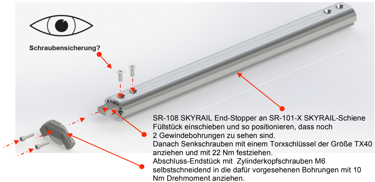
Abb. 3: Montage End Stopper SR-108
