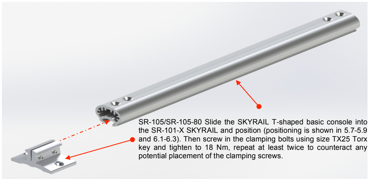
Fig. 1 Installation of SR-105 basic console
