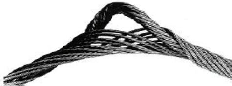
Figure 20, Core Protrusion, Indicating Shock Loading
