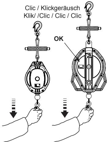
Check the locking of the lanyards by pulling sharply on the end (see chapter 3).
